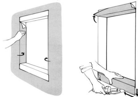
**For best result , extra heating and pressing is necessary to secure a good bonding at overlapping areas.**
